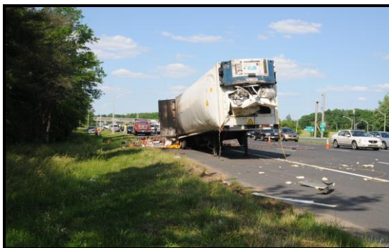
Figure 1 - Front of trailer damage to Refrigeration Unit
